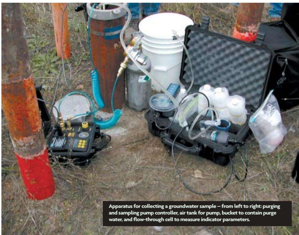
Apparatus for collecting a groundwater sample – from left to right: purging and sampling pump controller, air tank for pump, bucket to contain purge water, and flow-through cell to measure indicator parameters.
