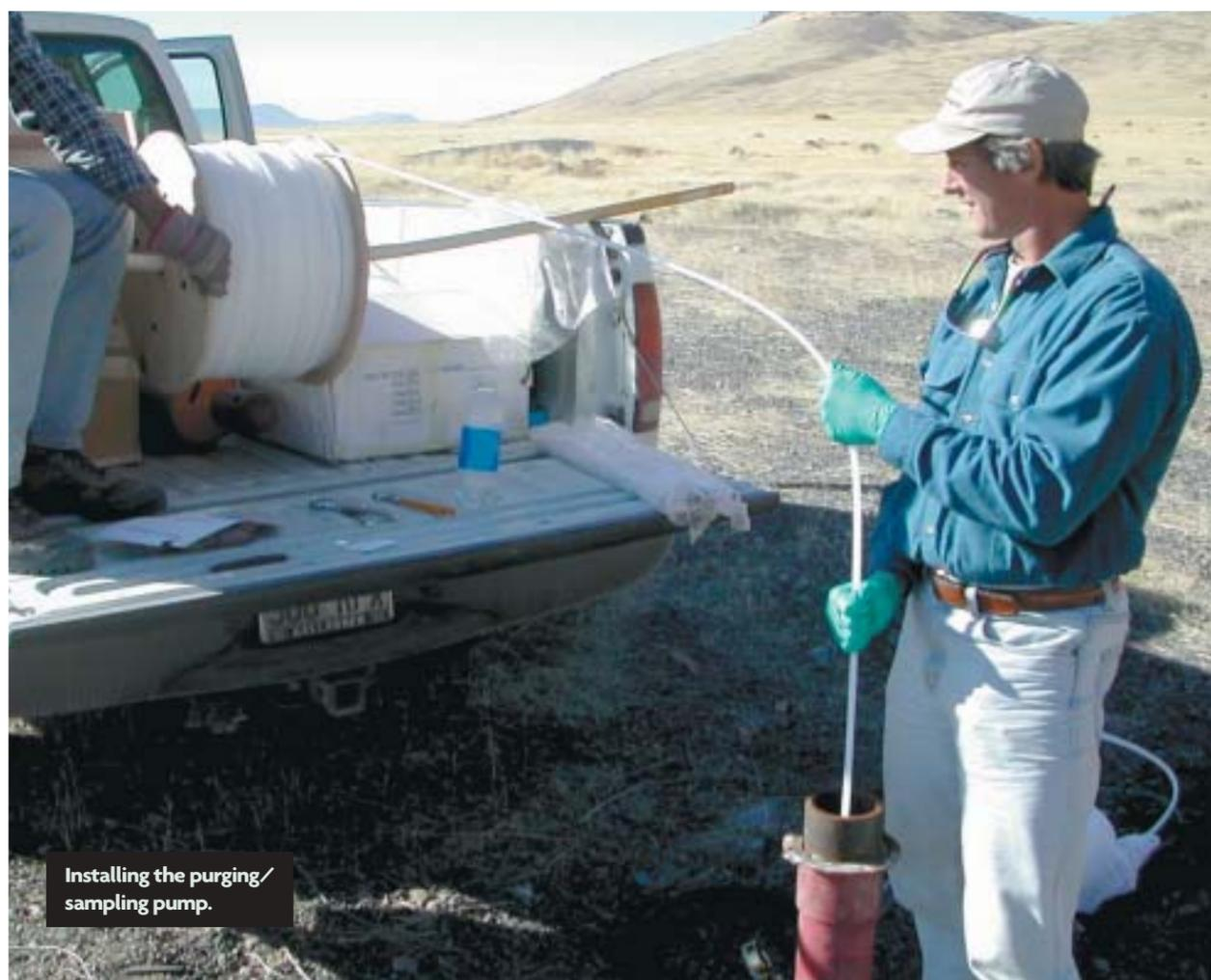
Installing the purging/sampling pump.
